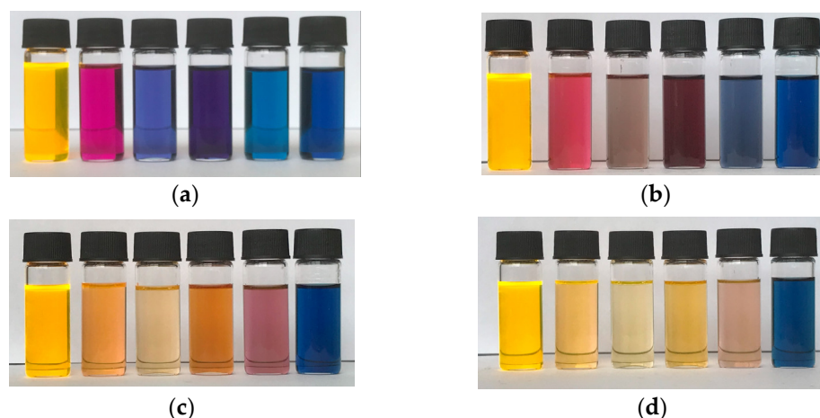
Figure 11. Behavior of PDI A and its thionated derivatives (from left to right: PDI A , PDI-1S , PDI-2S-cis , PDI-2S-trans , PDI-3S , PDI-4S ) in dichloromethane under sunlight in a saturated oxygen atmosphere: (a) t = 0 ; (b) t = 2 h; (c) t = 24 h; (d) t = 90 h.
