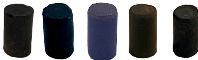
Figure 2. Representative photos of compressional cylinders of (from left to right) LOS 80 @230, LOS 85 @230, LOS 90 @230, LOS 90 @250, and LOS 90 @300.
