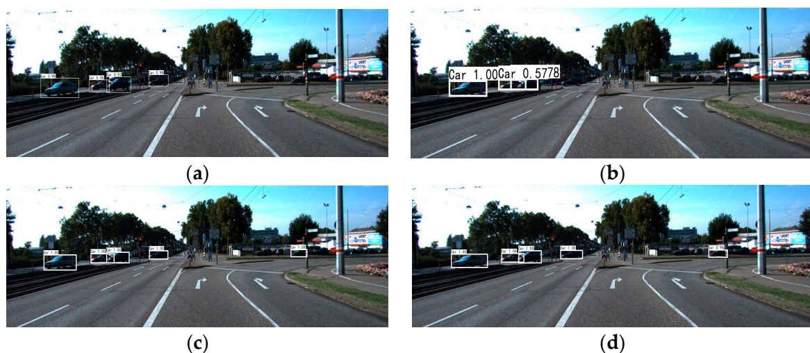
Figure 9. Low-light scenes. (a) Faster R-CNN detection effect, (b) SSD detection effect, (c) YOLOv3 detection effect, (d) MobileNetv2_CA detection effect.
