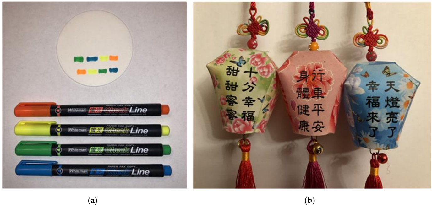
Figure 1. (a) Highlighter color pens and white filter papers used for chromatography experiments.; (b) decorative lights with randomly blinking LEDs used for dynamic colorimetric image analysis.
