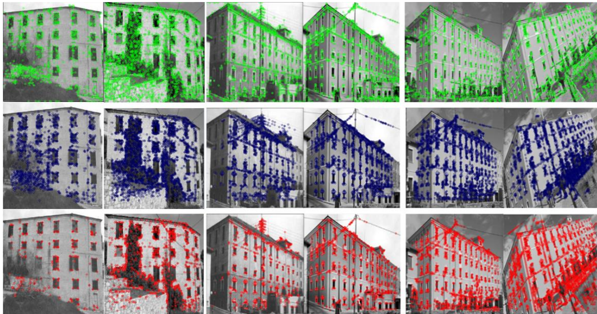
Figure 12. Tobacco industry building: detection of keypoints. The first pair of buildings is historic (1990–1992), the second pair has 20 years of distance (2000–2021), while the third pair of buildings is modern and of the same year (2022). Green, blue, and red keypoints indicate SIFT, ORB, and BRISK algorithms, respectively.
