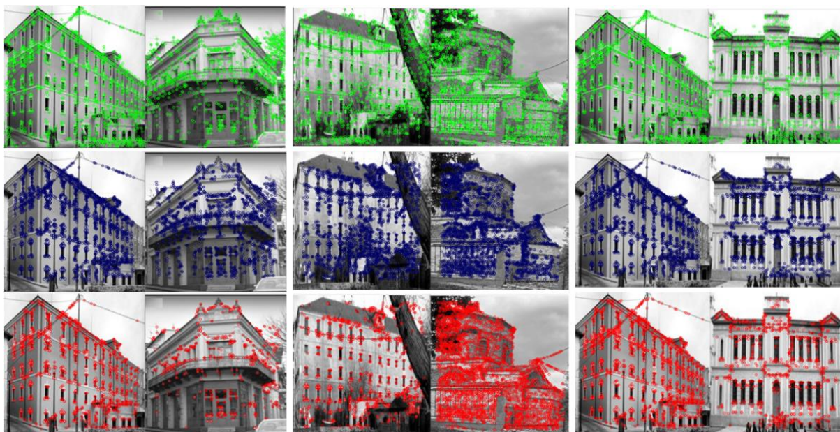
Figure 13. Keypoints detected by SIFT (green), ORB (blue), and BRISK (red) algorithms between different buildings. The first column includes two modern buildings. The second column includes two stone buildings, and the third column includes two buildings of the same order and at the same time; one is historical and the other modern.
