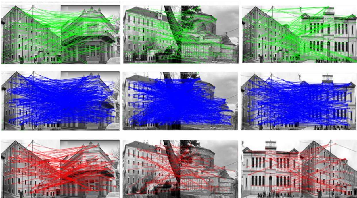
Figure 15. Feature matching of different buildings by SIFT, ORB, and BRISK algorithms with modified parameters.
