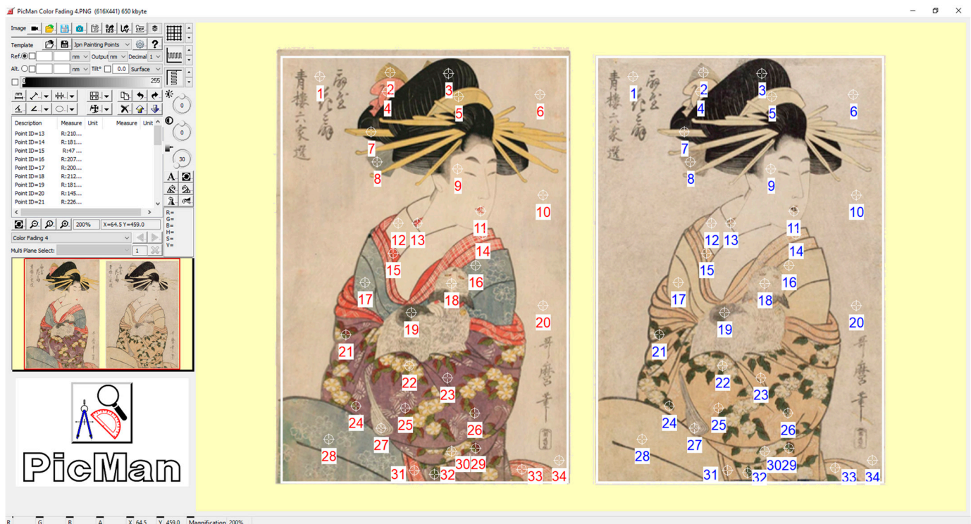
Figure 2. A screenshot image of image analysis software (PicMan) for color information extraction at 34 points of five-pixel diameter regions of interest (ROIs) and a 284 \times 422 pixel (= 119,848 pixels) rectangle (white border line) area per print. For easy comparisons, different colors for the numbers of ROIs for two images were used.
