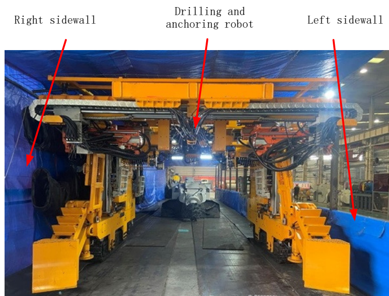
Figure 15. Drilling and anchoring robot test platform.
