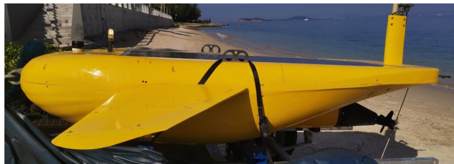
Figure 1. A specially shaped AUV equipped with a vectored thruster.
