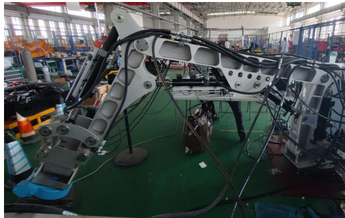
Figure 28. 7-DOFs rescue hydraulic robotic arm prototype.
