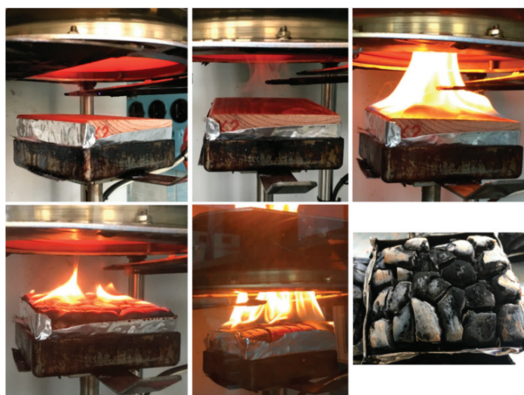
Figure 3. Samples tested in the cone calorimeter.
