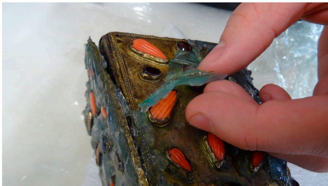
Figure 1. The gun from the Pierre Loti Museum collection (a), removal of the agar gel (b) (© J.G. Aubert/Arc'Antique—Grand Patrimoine de Loire Atlantique, Nantes, France).
