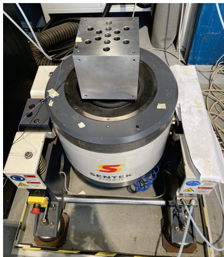
Figure 23. Head expander used for the X and Y tests.
