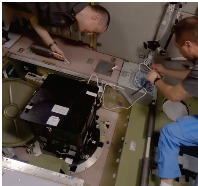
Figure 3. Mini-EUSO installed by two cosmonauts on the UV-transparent window of the Zvezda module.
