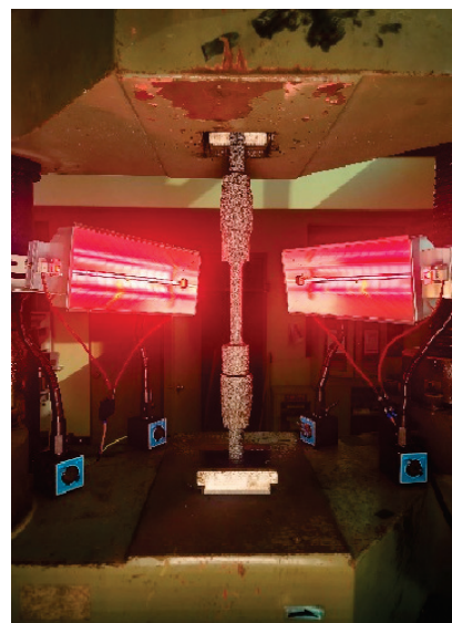
Figure 6. SMA bar heating tensile test.
