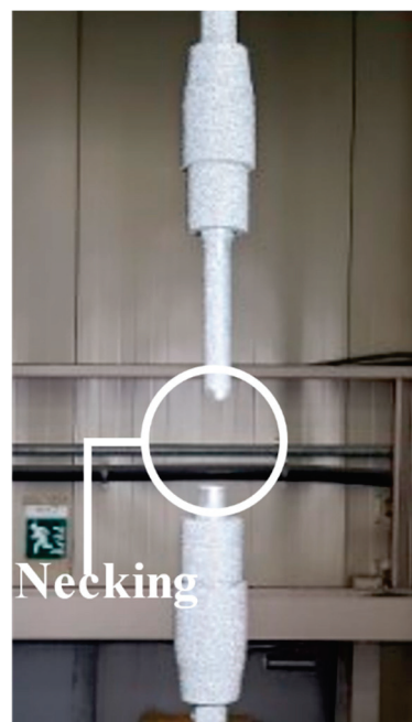
Figure 14. Failure shape of the SMA bar coupled with the D25 steel bar.
