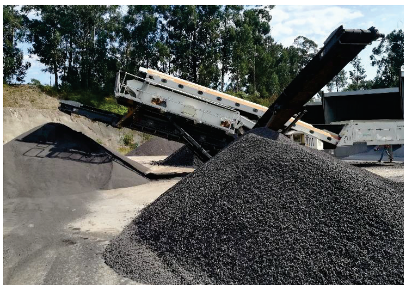
Figure 1. Steel slag aggregates from electric arc furnaces (EAF SSA).
