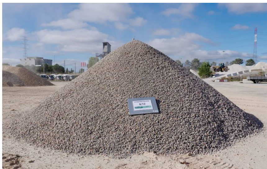
Figure 4. Recycled concrete aggregate (RCA) resulting from CDW processing.
