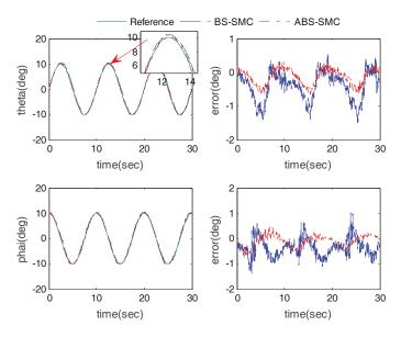
Figure 7. Robot end-effector angle tracking results (without subject).
