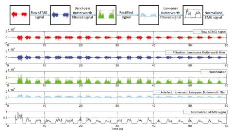
Figure 5. Surface electromyography (sEMG) signals after each processed step.
