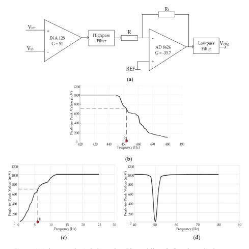
Figure 6. (a) is the system electrical schema of amplifiers and filters, (b-d) are the amplitude-versus-frequency curves of low-pass filter with the cut-off frequency  $f_L$ , and notch filter of 50 Hz, respectively.
