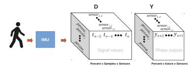
**Figure 3.** This figure illustrates how the matrix D was created. Every sample in the inertial measurement unit (IMU) is delayed by n times (in this case five times). The output matrix is shifted n times into the future (in this case three times).
