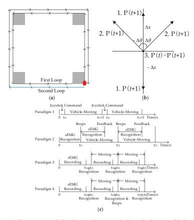
**Figure 5.** (a) Environment and obstacle maps. It contains the forward information (black vectors), backward information (blue vectors), starting point (red circle) and obstacle location (gray areas); (b) Three possibilities of the location update for Paradigm 1 and 2 ('1' denotes the straight-line movements, '2' denotes the rotation movements, and '3' is no movements); (c) The protocol for each paradigm. The onset of each real-time session is presented as the reference time point of 0 s.
