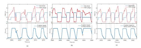
**Figure 11.** *M* variation during gait cycle. (**a**) variation of M during a gait test, which generates four sub-phases: initial contact (IC), mid-stance (MS), terminal stance (TS) and swing (SW); (**b**) example with three sub-phases; (**c**) example that shows the variation of M during a gait cycle with noise.
