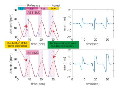
Figure 11. Actuator trajectory tracking results with abrupt disturbances.
