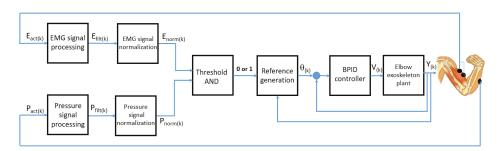
Figure 7. High-level control algorithm based on EMG and pressure signals for reference position generation.
