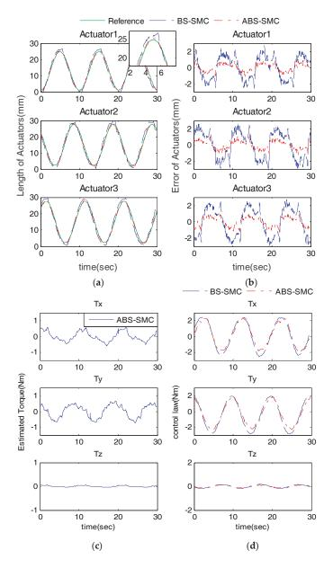
**Figure 8.** Actuator position tracking results with subject 1: (a) actuator position tracking results; (b) the actuator tracking errors; (c) the estimated external torque (using ABS-SMC) and (d) the control output tuning processing via ABS-SMC disturbance estimation.
