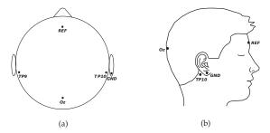
**Figure 1.** Positions on the scalp where the electrodes were located. (a) Top view of positions; (b) Side view of the positions. Oz: occipital area; TP9: left temporal area; TP10: right temporal area; REF: reference electrode; GND: ground electrode.
