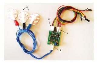
**Figure 3.** Surface electromyography (sEMG) circuit with two channels and the electrodes: 1—electrodes, 2—electrode connector, 3—connectors for power supply (5 V and GND), 4—connector for serial peripheral interface (SPI) communication.
