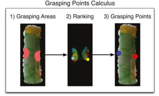
**Figure 4.** Steps of the method for calculating a pair of contact points. Scene Segmentation: clouds of the detected objects. Grasping Points Calculus, executed for each detected object: (1) grasping areas with potential contact points, (2) curvature values and a pair of evaluated contact points, (3) best ranked pair of contact points.
