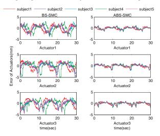
Figure 10. Actuator tracking error results with five subjects.
