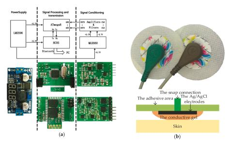
Figure 1. (a) The four-channel offline acquisition board; (b) The wet disc sensors and architecture.
