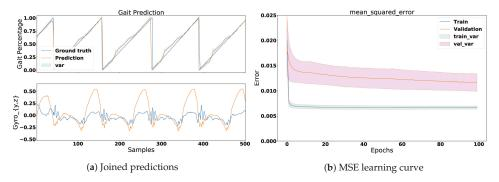
**Figure 8.** This figure shows the prediction and learning process results of the joined signal for several subjects. Similar to Figure 7, (a) shows the comparison between the prediction and the ground truth and (b) illustrates the learning curve of the MSE. The average MSE reached a loss of 0.006 in the training set and an average of 0.0115 in the test set.
