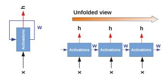
**Figure 2.** This figure illustrates the information flow in a recurrent neural network (RNN). The left image shows an RNN as an infinite loop network where the model outputs are fed back as inputs. The right figure is an unfolded representation of an RNN [53].
