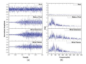
**Figure 7.** Time-frequency verification of different movements: (a) Normalized amplitudes in time domain; (b) PSD in frequency domain. (The names of four movements were represented to their abbreviations in the following analysis)
