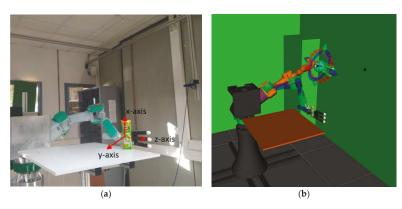
**Figure 1.** Pre-grasping pose of the robotic system computed by the vision algorithm. (a) Real robotic system in which the grasps are executed. (b) Simulation system where the movement is planned and the robotic hand pose is evaluated.
