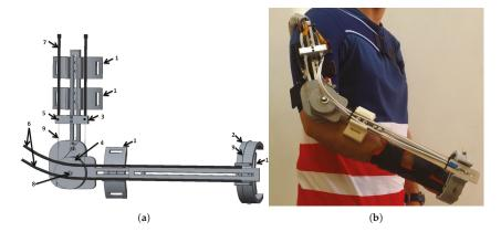
**Figure 2.** SMA exoskeleton design. **(a)** CAD structure: 1—attachment points with the hand and force-sensing resistor (FSR) sensors, 2—fixed structure for supination–pronation, 3—actuator termination for Bowden tube, 4—pulley for linear to rotational transformation, 5—temperature sensors, 6—supination–pronation actuators, 7—flexion–extension actuators, 8—absolute encoder, 9—SMA wires. **(b)** SMA elbow joint exoskeleton on a human body.
