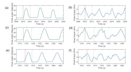
**Figure 12.** Knee angle and knee torque during knee impedance modulation with patterns  $G: P_1(\mathbf{a}, \mathbf{b}); P_2(\mathbf{c}, \mathbf{d}); P_3(\mathbf{e}, \mathbf{f}).$
