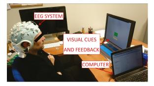
**Figure 2.** Experimental setup. Subjects sat looking at a screen which fed them with instructions while their EEG signals were recorded. Furthermore, the screen gave feedback about their performance in each task. The participant in the picture gave written informed consent to publish the image.
