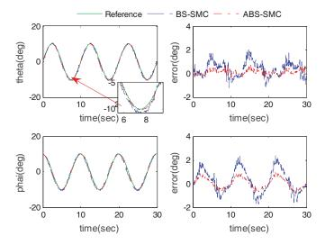
Figure 9. End-effector angle tracking results with subject 1.
