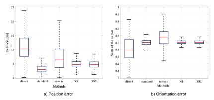
**Figure 5.** Position and orientation errors using different calibration methods: (a) Position error measured as a distance from the correct position; (b) Norm of the orientation error vector computed by Rodrigues' expression.
