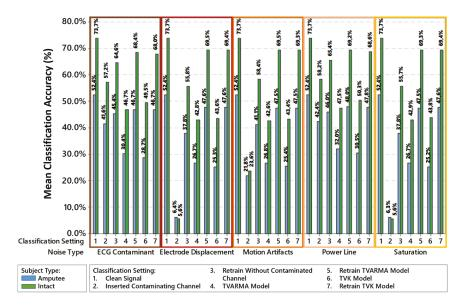
**Figure 6.** Classification setting comparison for each contaminant insertion type and the clean sEMG signal classification.
