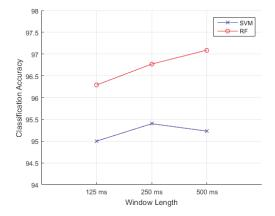
**Figure 10.** Effect of window length on the classification accuracy. The classification accuracies are averaged over all nine subjects.
