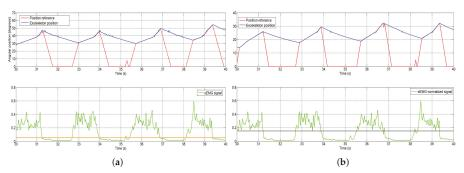
**Figure 6.** (a) the orange line shows data using a 0.05 threshold. (b) the black line shows data using a 0.15 threshold.
