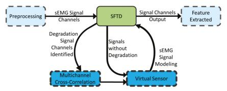
Figure 5. The operating logic of the SFTD with the virtual sensor.
