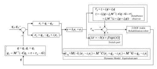
Figure 4. Implementation of ABS-SMC for the ankle rehabilitation robot.
