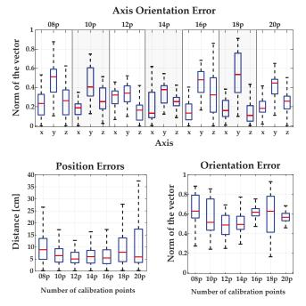
**Figure A3.** Results obtained by the RANSAC calibration method using different numbers of calibration points.
