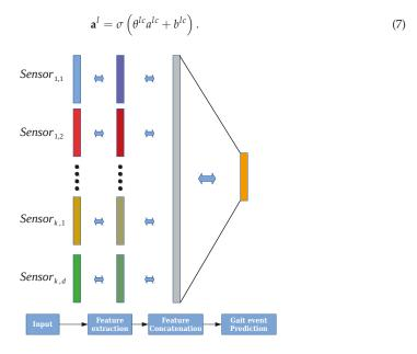
**Figure 4.** This figure illustrates the exponentially delayed fully connected neural network (ED-FNN) architecture. Initially, the network individually receives each sensor input from the matrix X in Equation (5). Then, the network separately extracts the features of each sensor and concatenates them into a single feature vector. Finally, the output layer uses the feature vector to forecast the gait events of the cycle.
