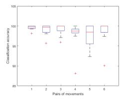
**Figure 8.** Boxplot for EMG tasks classification accuracy with ECU and ECR. The horizontal axis represents the different pairs of movements (1: REST vs. MF, 2: REST vs. WE; 3: REST vs. WF, 4: MF vs. WE, 5: MF vs. WF, and 6: WE vs. WF).
