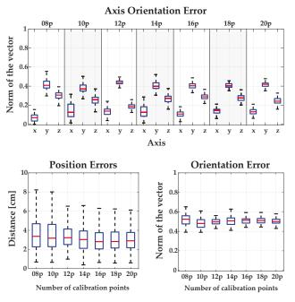
**Figure A2.** Results obtained by the standard calibration method using different numbers of calibration points.
