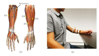
Figure 3. Sensor placement and implementation of the system. (a) Sensor placement in the offline analysis and the pairs of yellow points correspond to the bi-polar electrodes; (b) Real-time system setup for data acquisition.
