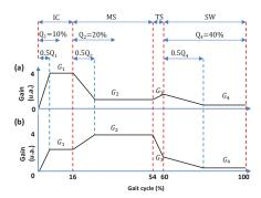
**Figure 3.** Percentage of each phase with respect to the gait cycle  $(Q_i)$  taken into account in this approach for (a) gain pattern  $P_1$ ; (b) gain pattern  $P_2$ .
