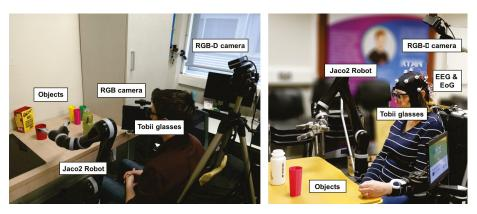
**Figure 1.** AIDE system integrates three different hardware modules: (i) a full-arm robotic exoskeleton or a Jaco2 robot; (ii) multimodal interfaces, consisting of a pair of gaze-tracking glasses (Tobii glasses) and a hybrid brain–computer interface (BCI) based on electroencephalography (EEG) and electrooculography (EOG); and (iii) context recognition sensors: a RGB-D camera to locate the object's pose and a camera to compute the user's head and mouth pose.
