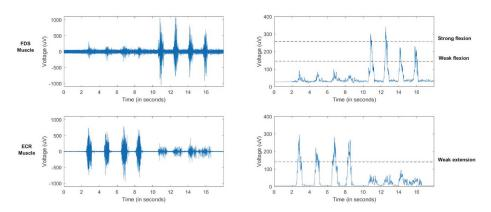
**Figure 3.** EMG raw signal for several flexion/extension wrist movements (**left**). Processed EMG signal and estimative thresholds (**right**).
