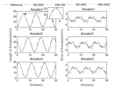
Figure 6. Actuator position tracking results (without subject).
