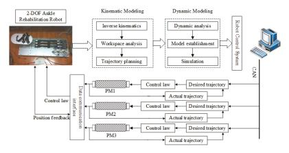
Figure 1. System structure of the ankle rehabilitation robot.
