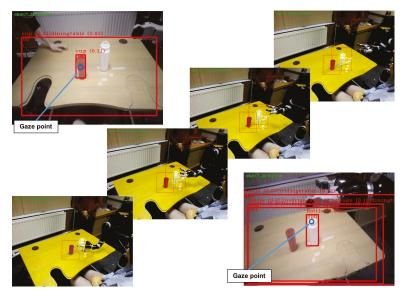
**Figure 10.** Images of the context recognition and eye-tracking systems in experimental tests. Examples of object detection (cup and bottle) with the estimated gaze position (blue circle). Snapshots of the experiments: grasping a bottle using the Jaco2 robot.
