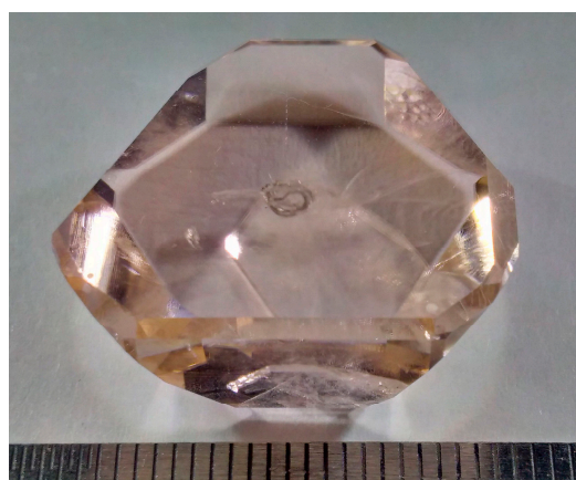
Figure 1. As-grown Er,Yb:GdMgB 5 O 10 single crystal.
