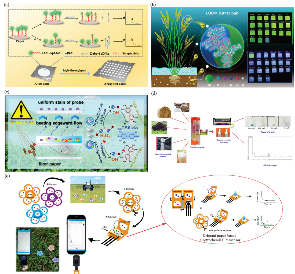
Figure 8. (a) Illustration of a high-throughput paper-based FRET aptasensor designed for the detection of Pb 2+ . Reprinted with permission from Suo et al. [187]. ©2022 Elsevier B.V. (b) Schematics of fiber-made filter-paper-based biosensors for the real-time monitoring of Cd 2+ in water, rice, and rice soil. Reprinted with permission from Yu et al. [188]. ©2023 American Chemical Society. (c) Principle illustration of the paper-based colorimetric sensor for real-time monitoring of pesticides. Reprinted with permission from Zhang et al. [193] ©2022 Elsevier B.V. (d) Schematic illustration of pesticide detection in dairy samples using the paper-based sensor. Reprinted from Ranveer et al. [194] under a Creative Commons license ©2022 Elsevier B.V. (e) Schematic representation of the origami paper-based electrochemical biosensor for pesticide detection. Reprinted with permission from Caratelli et al. [195]. ©2022 Elsevier B.V.
