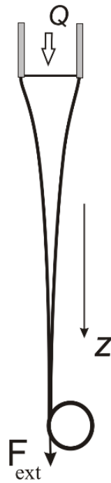
Figure 13. Stretching of a polymer solution jet by an external force F_{ext} during continuous fiber spinning.
