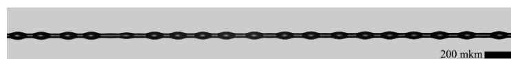
Figure 14. Blistering structure formed by continuous drawing out of a 25% solution of PAN ( M_w = 85,000 ) in DMSO. Authors' photo.
