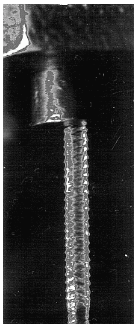
Figure 9. Self-oscillations at the exit of a capillary.
