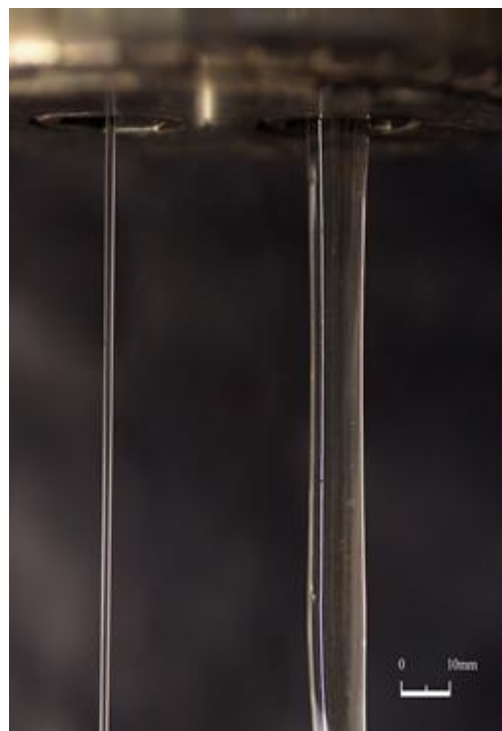
Figure 7. Comparison of two jets obtained at the same volume output but with different lengths of capillaries, long (left) and short (right), authors' photo.
