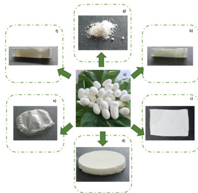
Figure 24. Representation of the instances of BINMs in devices fabricated by processing silkworm cocoons (a) for wound healing application: fibroin hydrogel (b), electrospun fibroin (c), sponge (d), film (e), solution (f), and powder (g). Reprinted with permission from Ref. [381].
