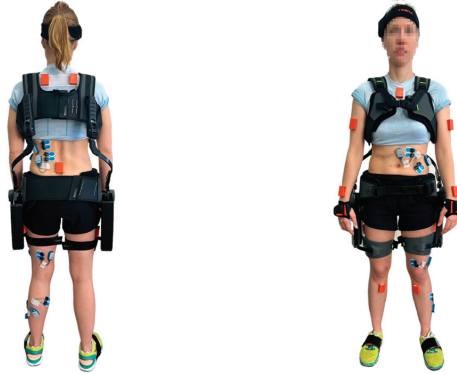
Figure 4. Sensor placement of sEMG and Xsens sensors.
