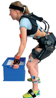
Figure 1. Task 1: lifting and lowering a box with the exoskeleton PaexoBack.
