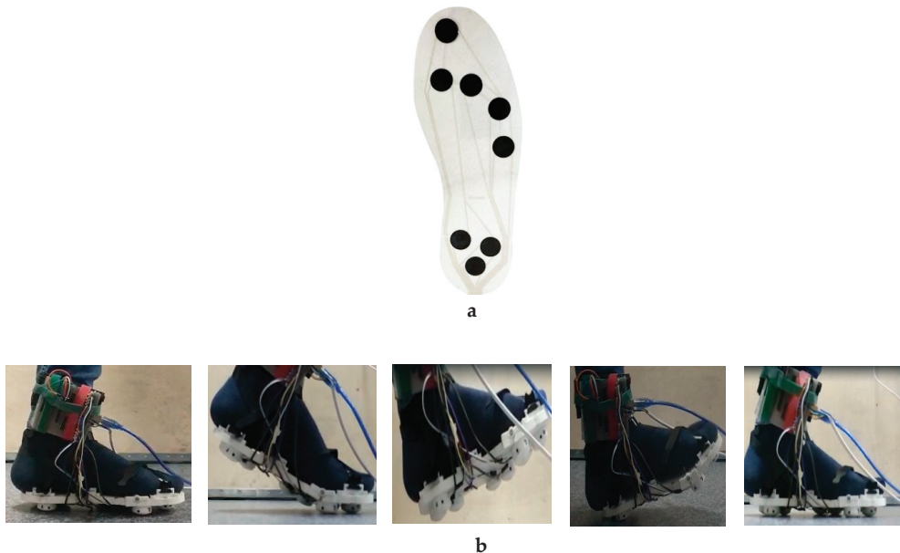
Figure 5. (a) Distribution of pressure sensors on the sole; (b) one-legged stepping cycle.
