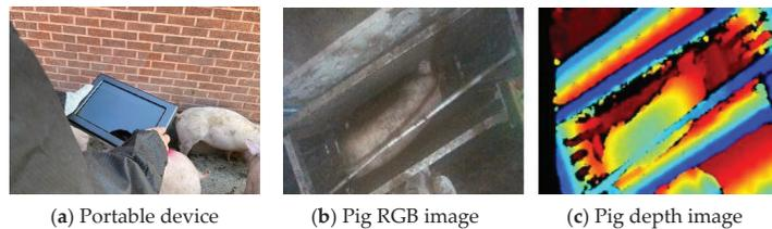
Figure 1. Developed portable device and color and depth images for pigs in a field.
