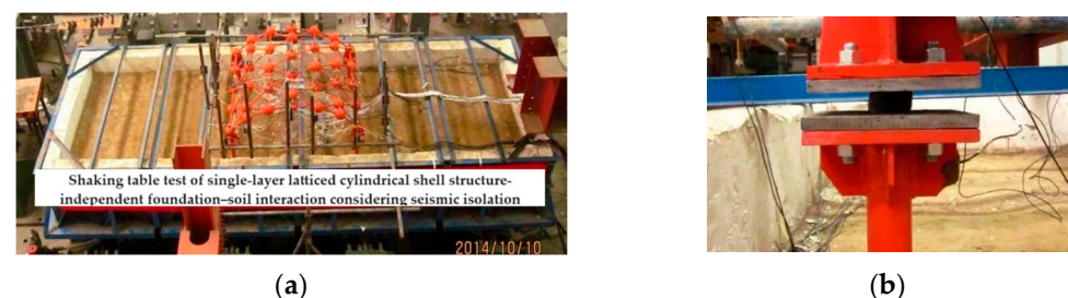
Figure 22. Shaking table test of single-layer latticed cylindrical shell structure-independent foundation–soil interaction considering seismic isolation [16]: (a) soil container with experimental model; (b) layered rubber bearing and its connection.
