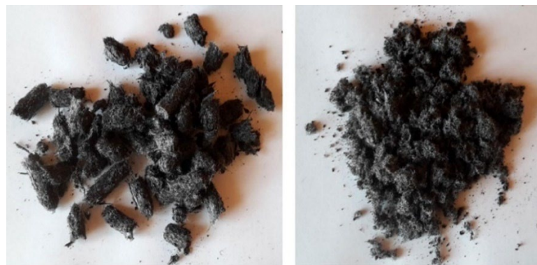
Figure 12. Fiber pellets obtained with (left) and without (right) paraffin wax [10].
