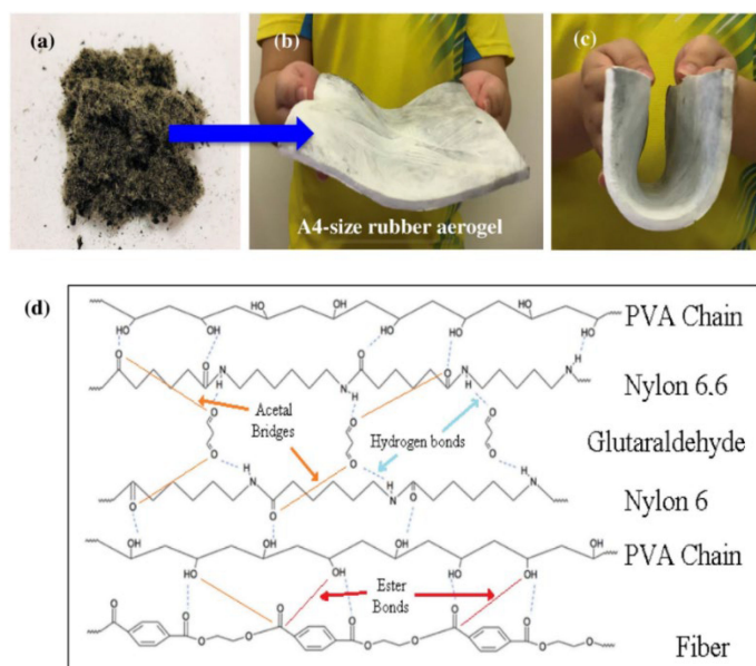
Figure 14. (a) Raw WTTF obtained from shredding the car tire waste, (b) A4-size rubber aerogel, (c) high flexibility of the rubber aerogel and (d) proposed formation mechanism between the WTTF and the crosslinkers inside the rubber aerogel [109].
