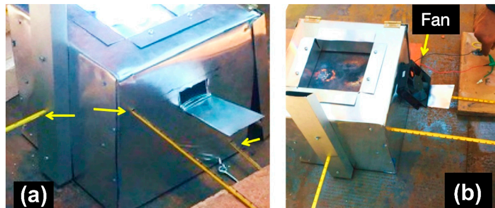
Figure 6. (a) Location of the thermocouples (indicated with yellow arrows). (b) Location of fan.
