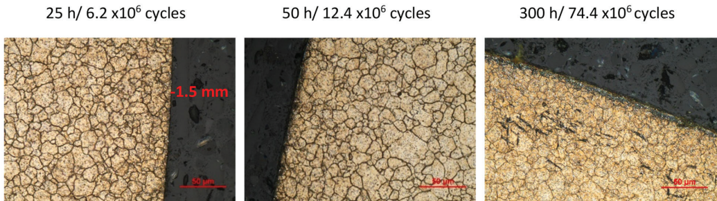
Figure 6. Cross-sectional cuts and metallographic examination of the rollers run with the high ref oil.
