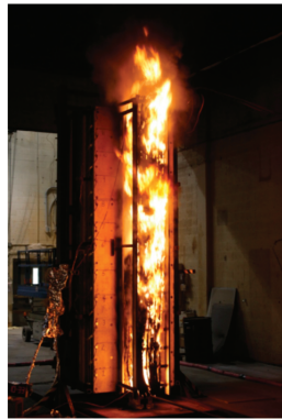
Figure 31. Cable tray fire. Refs. [181,182].
