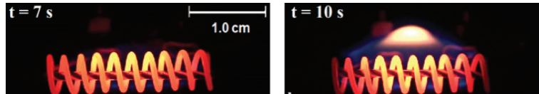
Figure 1. Ignition phenomenon of the NiCr-PE wire ( d_c = 0.7 mm, \delta_p = 0.15 mm). Reprinted from Ref. [15] with the permission of Elsevier.
