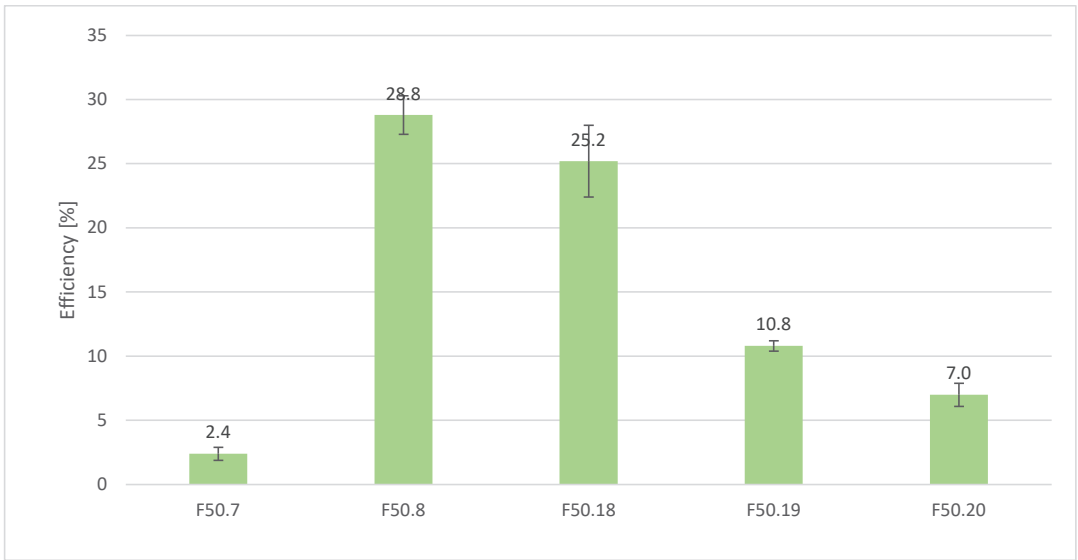
Figure 6. The efficiency of the formulations F50.7 ( \text{Mg}(\text{OH})_2 = 130 ; \text{PCC} = 0 ), F50.8 ( \text{Mg}(\text{OH})_2 = 40 ; \text{PCC} = 90 ), F50.18 ( \text{Mg}(\text{OH})_2 = 30 ; \text{PCC} = 100 ), F50.19 ( \text{Mg}(\text{OH})_2 = 90 ; \text{PCC} = 40 ), F50.20 ( \text{Mg}(\text{OH})_2 = 100 ; \text{PCC} = 30 ). Standard deviation ranges are reported.
