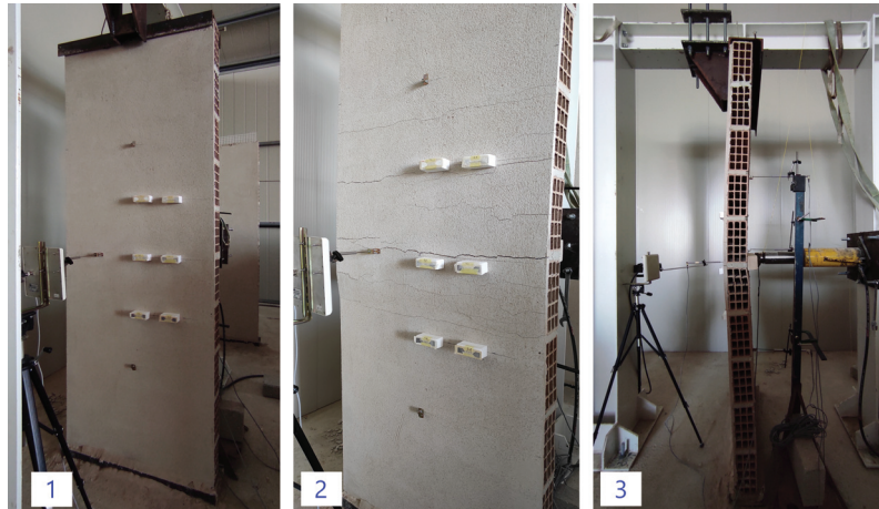
Figure 28. In situ experimental test conducted on the 1st wall: (1) Set-up; (2) first deformations and cracks; (3) Maximum deformation reached at 60 mm of displacement.
