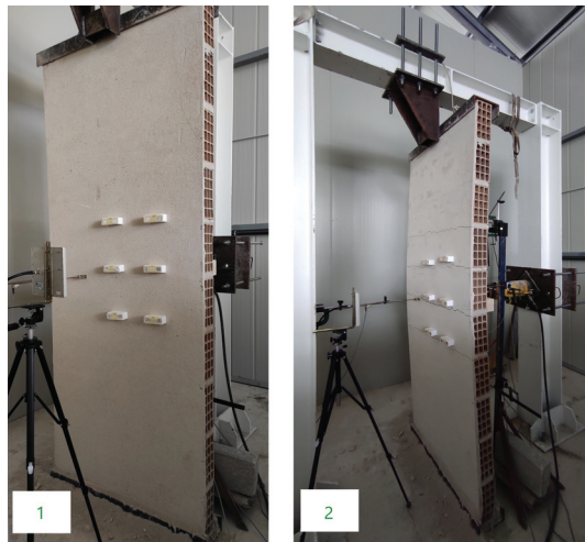
Figure 29. In situ experimental test conducted on the 2nd wall: (1) Set-up; (2) Complete deformation of the wall in correspondence of the final displacement of 70 mm.
