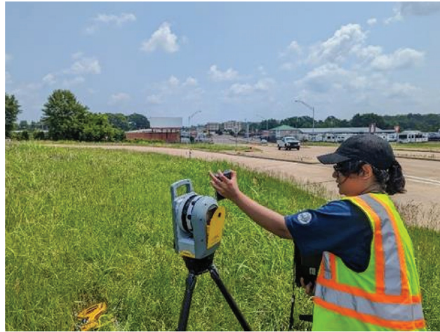
Figure 5. LiDAR survey conducted on the site.
