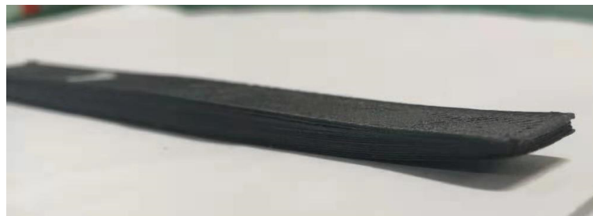
Figure 11. Printed samples (warpage deformation).
