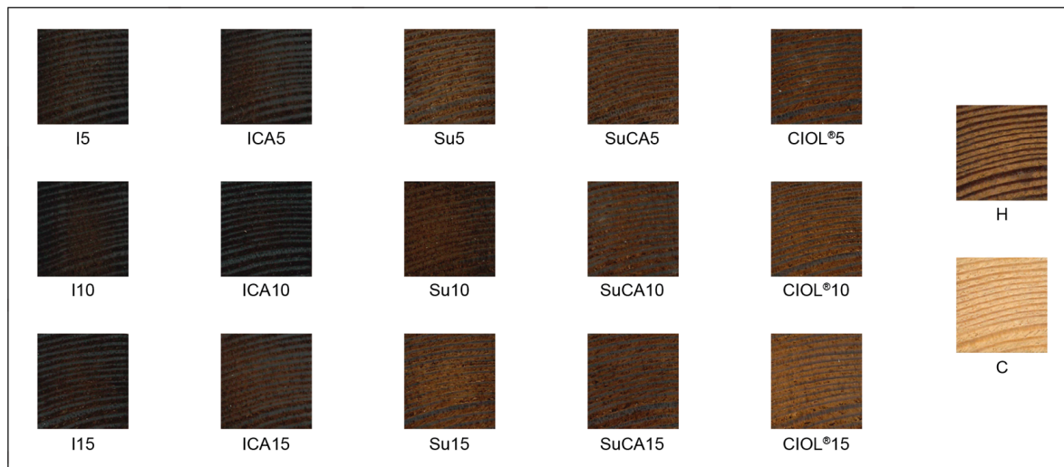
Figure 3. Cross-sectional appearance of specimens after heat treatment and the untreated control (C).
