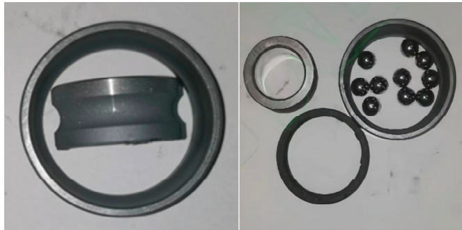
Figure 4. Bearing with MoS 2 coating.
