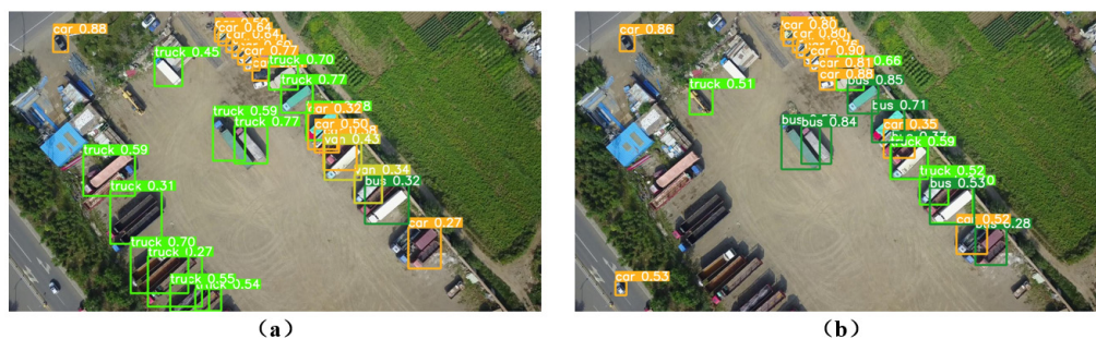
Figure 9. Schematic diagram of the detection results of two backbone networks (a) and three backbone networks (b) in the composite backbone network. From the comparison of the two figures, the number of targets detected in (b) is significantly less than in (a), which proves that the effect of the two backbone networks in the composite backbone network is better than that of the three backbone networks.
