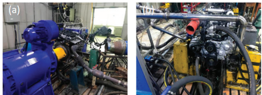
Figure 2. Engine bench test device diagram. (a) Engine's testing bench. (b) The CA4D28C5 diesel engine testing device.
