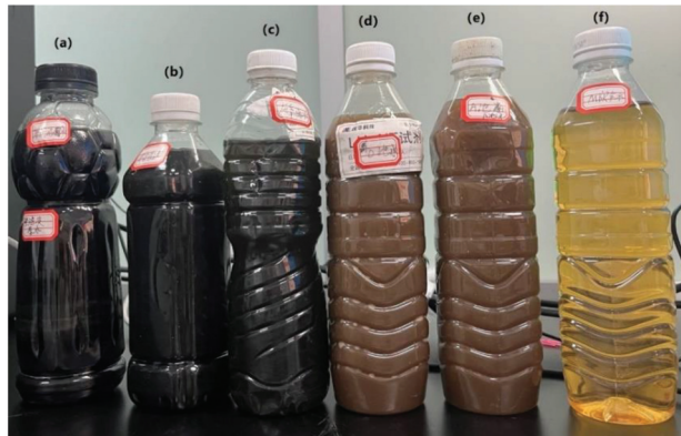
Figure 2. Leachate sample collection: (a) leachate raw water (LRW), (b) leachate effluent (LE), (c) internal circulation reactor effluent (ICRE), (d) aerobic effluent (AeroE), (e) Anaerobic effluent (ANE), and (f) MBR effluent (MBRE).
