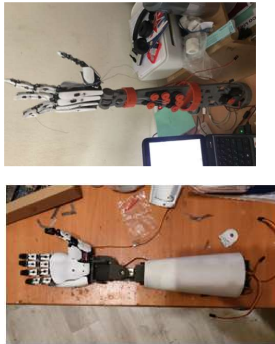
Figure 5. Engineered construction of an anthropomorphic robotic arm.
