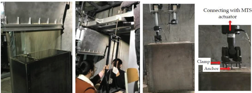
Figure 2. Sand preparation, installation and connection with actuator of anchors.
