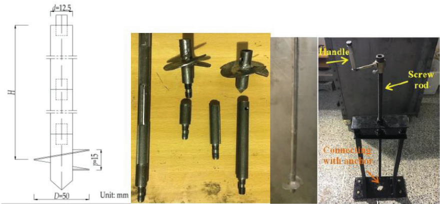
Figure 1. Model of helical anchor and torsion mounting frame.
