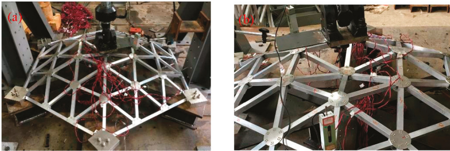
Figure 4. Failure patterns of the lattice shell model without aluminum alloy plates: (a) The overall failure profile; (b) The amplified profile of a local destabilization area.
