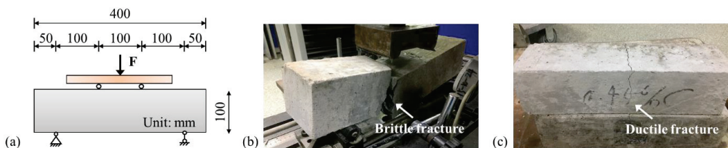
Figure 3. Loading and failure diagram of bending test: (a) loading diagram, (b) failure pattern of plain concrete; (c) failure pattern of FRC.
