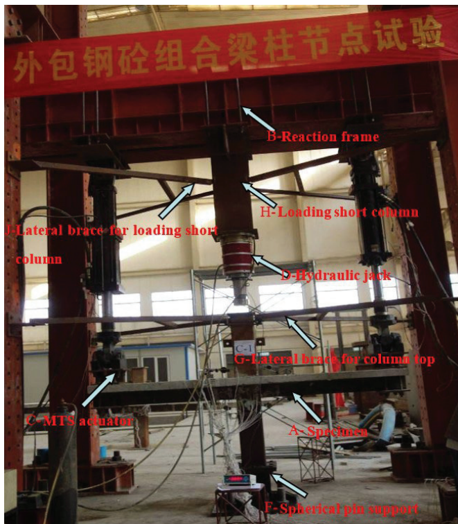
Figure 6. Test setup: (a) the schematic of the test setup; (b) test loading site.
