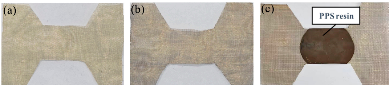
Figure 2. Resistance elements: (a) UT-RE, (b) Ox-RE, and (c) Ox-RE/PPS.
