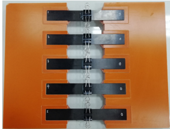
Figure 3. The fabricated single-lap specimen.
