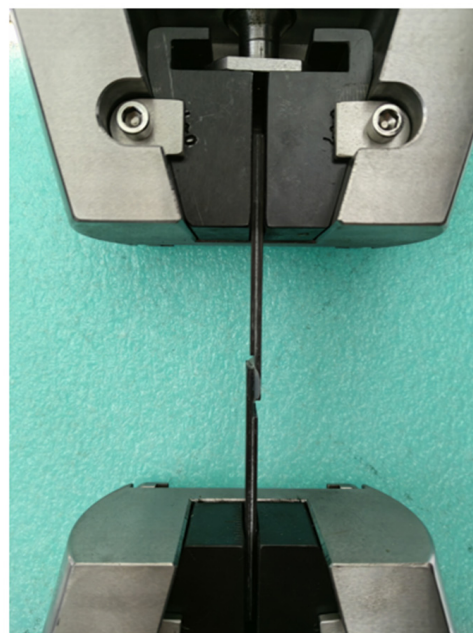
Figure 4. Tensile shear test of single-lap specimen.
