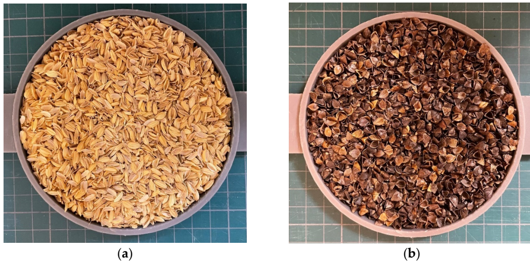
Figure 3. Samples for tortuosity measurement: (a) rice husks; (b) buckwheat husks.
