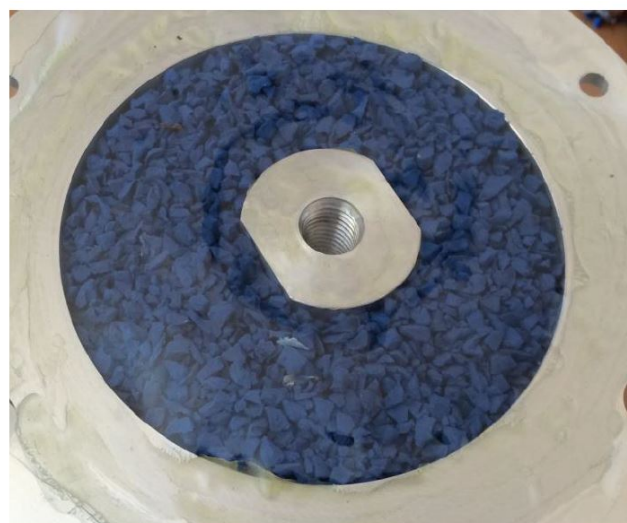
Figure 7. SVPP damper with EPDM grains.
