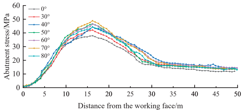
Figure 12. Abutment stress in front of the working face for different fault dip angles.
