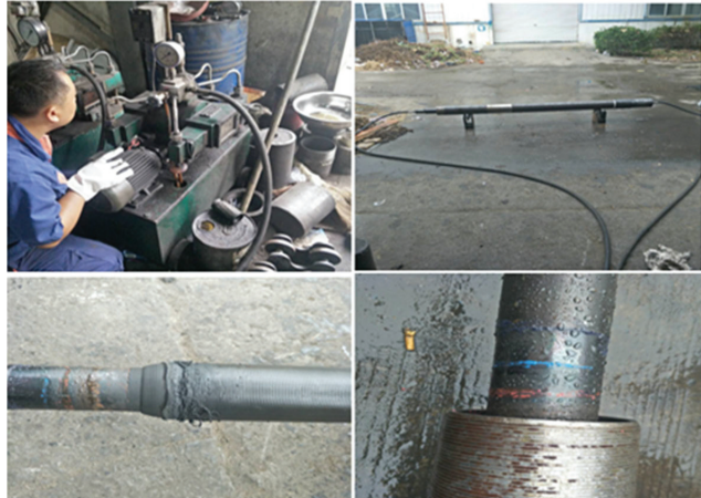
Figure 7. Reliability test of inflatable fracturing packer.
