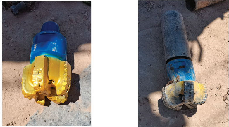
(a) The drill before use (PDC, \varnothing 215.9 mm) (b) The drill after use (PDC, \varnothing 215.9 mm)
