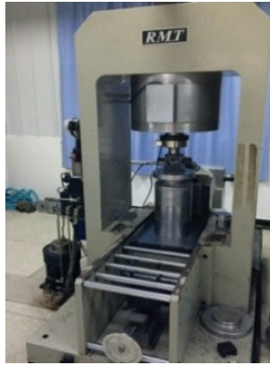
Figure 2. RMT-150C test system for rock mechanical properties.
