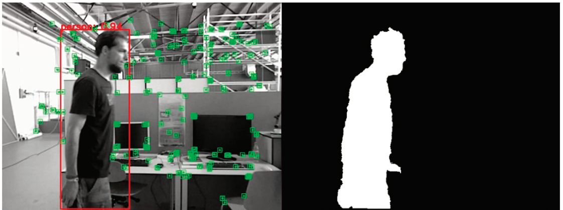
Figure 5. The result of semantic segmentation based on our method. The red represents the target detection box; the green represents static feature points in the keyframe. The depth value of white area is 1, while that of the black area is 0.
