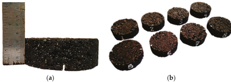
Figure 4. (a) Pre-notched sample; (b) Group of demoulded specimens.
