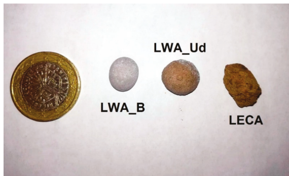
Figure 2. External shape of LWA_B (left), LWA_Ud (center) and LECA (right).
