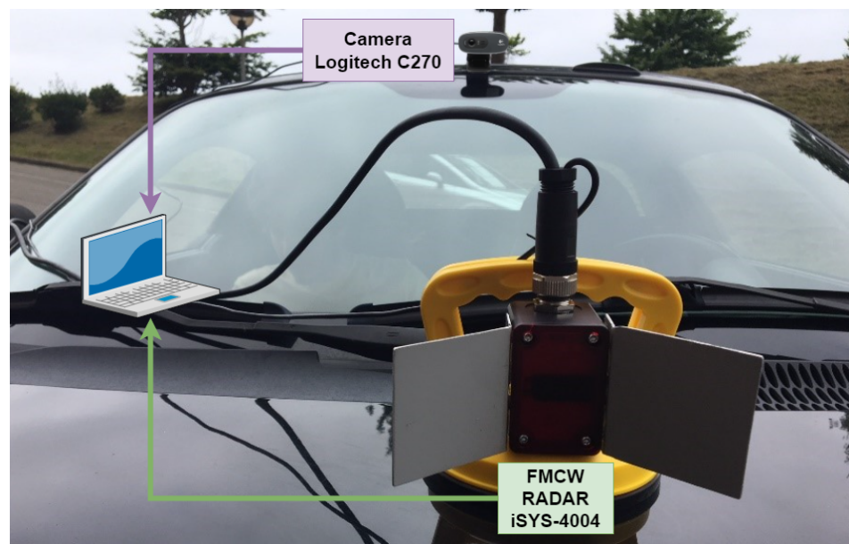
Figure 5. Mounting of the radar on the vehicle.
