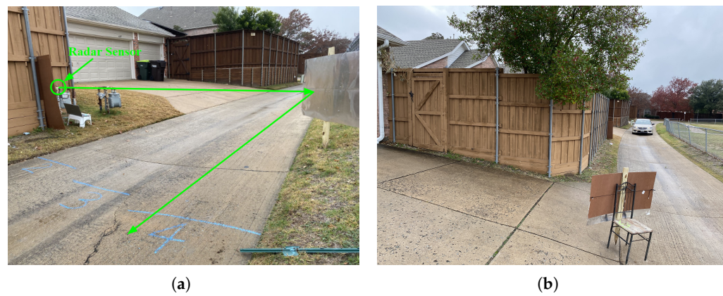
Figure 2. The setup of the reflector in (a) blind spot tests and (b) field simulation tests.
