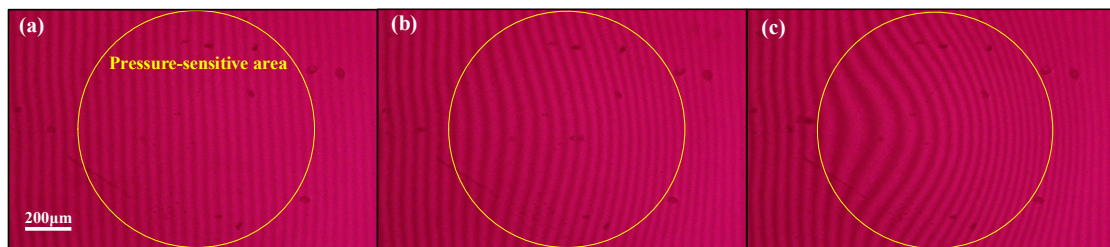
Figure 6. Images of interference patterns at pressure load of (a) 0 mmHg, (b) 22.5 mmHg, (c) 45 mmHg.
