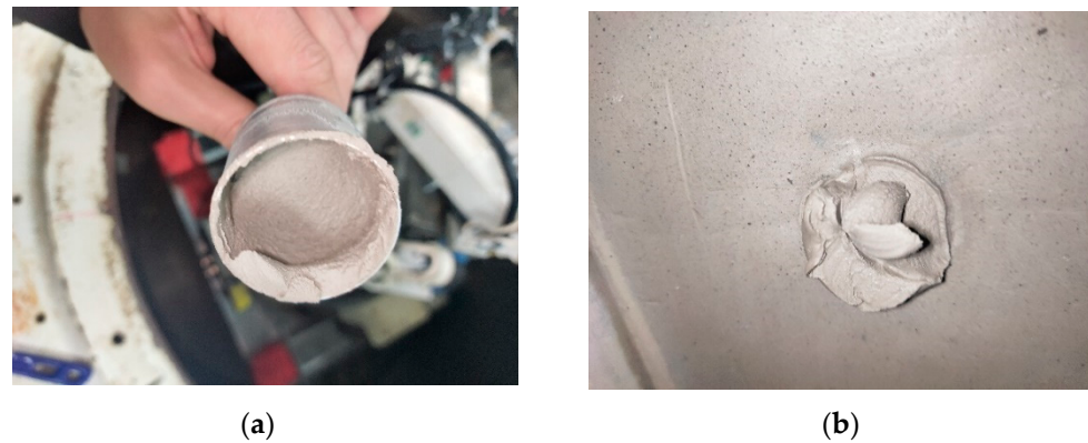
Figure 12. Soil plug inside bucket and soil surface after pull-out of bucket: (a) Soil plug inside bucket; (b) Soil surface after pull-out of bucket.
