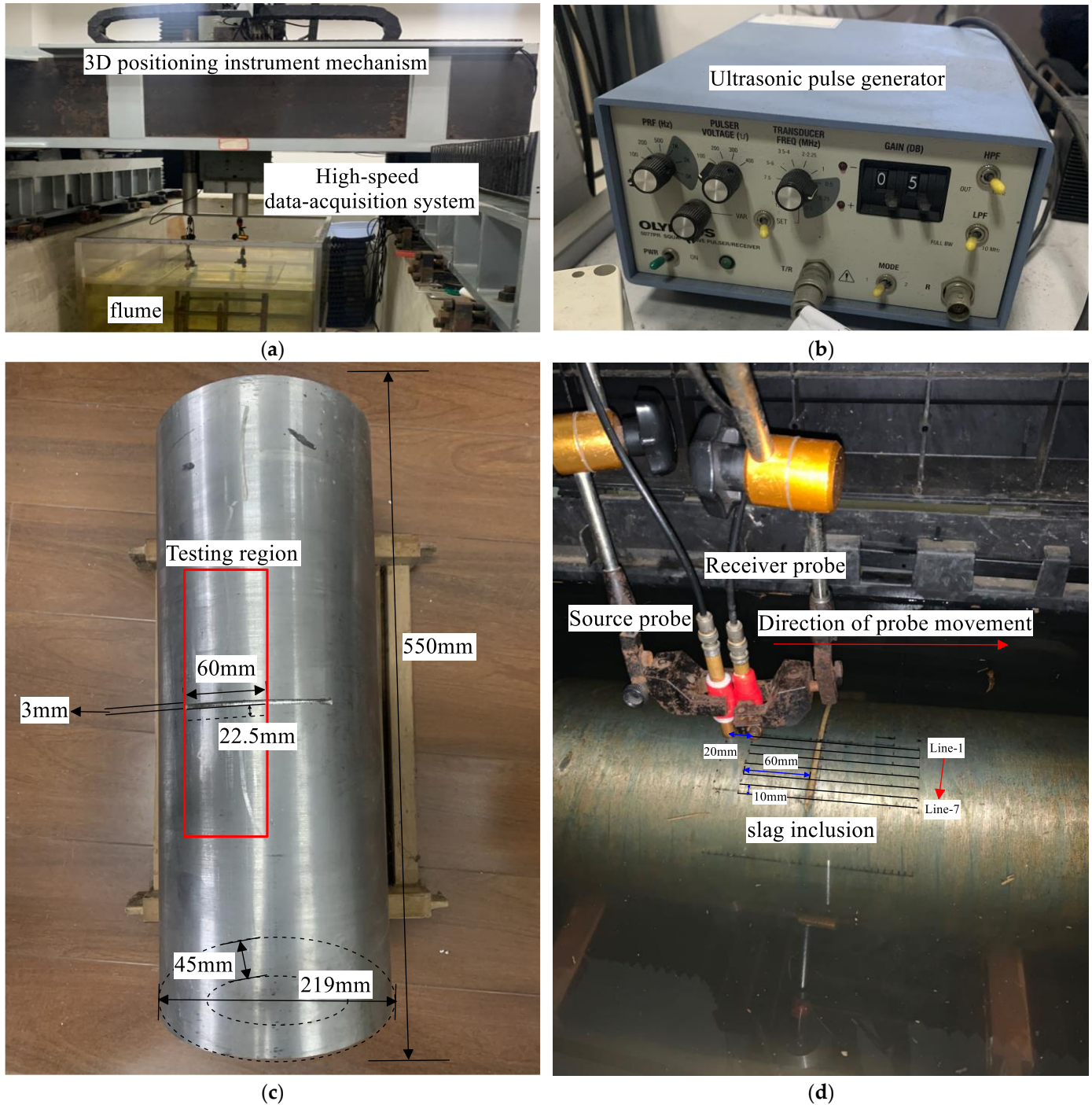
Figure 14. Ultrasonic experimental setup and observing system. (a) Three-dimensional positioning instrument mechanism; (b) Ultrasonic pulse generator; (c) Specimen; and (d) Observing system.
