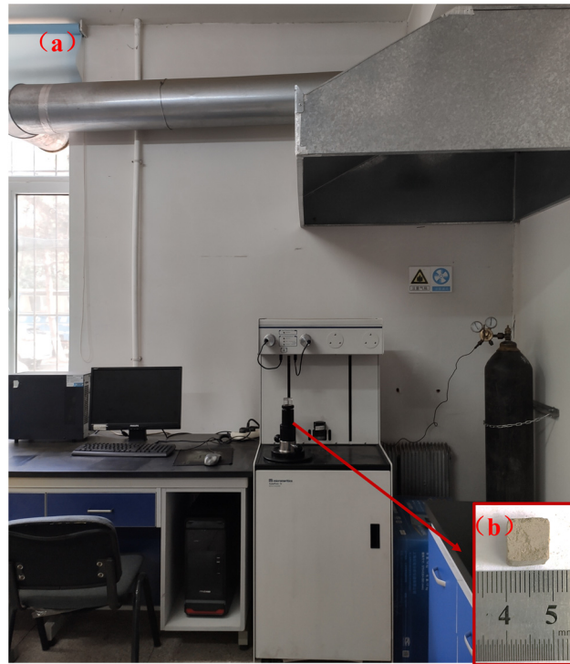
Figure 5. Instrument and sample for MIP and SEM test: (a) AutoPore IV 9500 Porosimeter; (b) the sample for the MIP test.
