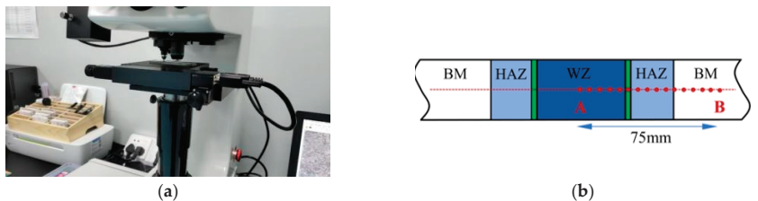
Figure 4. Hardness test. (a) Instrument for Vickers hardness test; (b) schematic diagram of the location of Vickers hardness measurement points.
