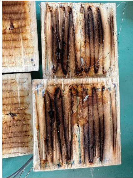
Figure 9. Stage III of tests in which failure occurs due to the thermal decomposition of the materials.
