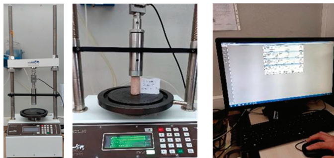
Figure 6. Triaxial strength test device and placing the sample on the device.
