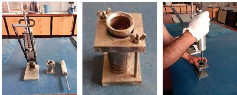
Figure 4. Specimen preparation with Harvard miniature compaction equipment.
