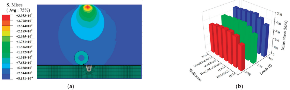
Figure 18. Mises stress distribution in the weld zone under different loads. (a) Mises stress distribution in the BM under 200 t. (b) Mises stress distribution in the welded joint under different loads.
