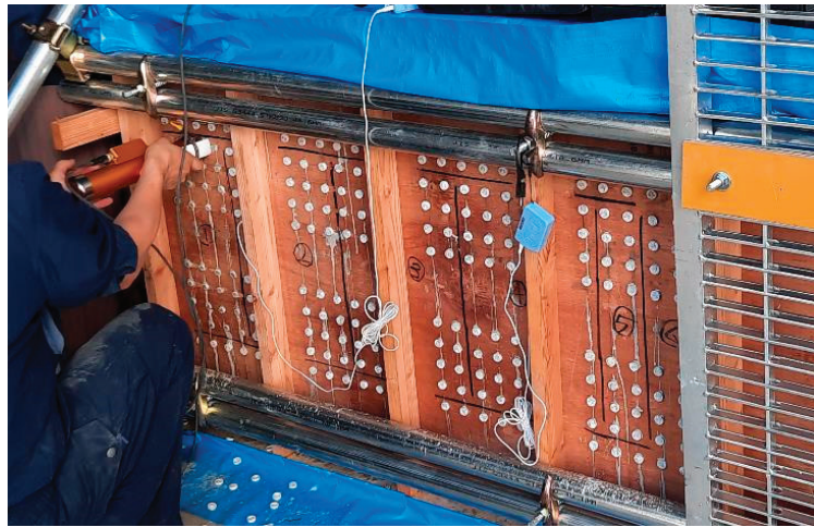
Figure 3. Pin penetration test of the mock-up mold before demolding.
