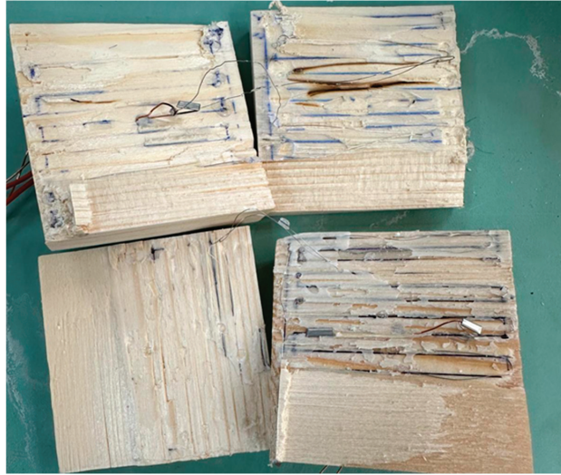
Figure 7. Stage I of tests in which failure occurs due to wood shearing parallel to the fibers.
