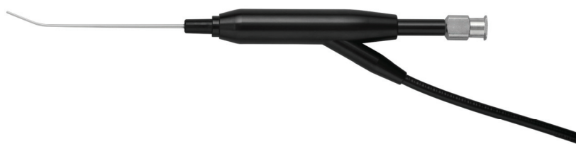
Figure 1. The MT-3000 dacryoadenoscope (FiberTech Co., Tokyo, Japan) used in this study. This device has a tapered tip and acquires low-quality images (3000 pixels). The probe length is 50 mm, the outer diameter of the root is 1.0 mm, and the outer diameter of the tip is 0.7 mm, with an angulation of 27° 10 mm from the tip.
