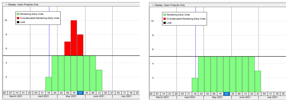
Figure 1. Resource allocation verification. Resource overallocation in the initial project plan, indicating potential issues during project execution (a). The schedule generated by Optimizoo, demonstrating improved resource allocation for a more efficient and feasible execution plan (b).
