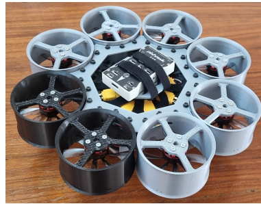
Figure 16. Top view of the octorotor mini-UAV manufactured fuselage.
