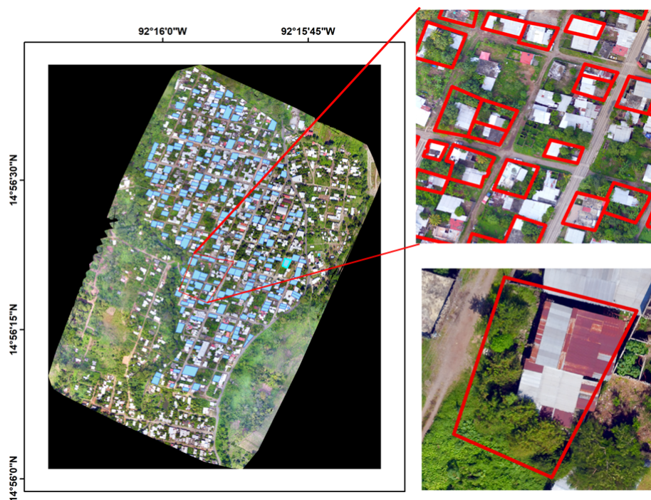
Figure 1. Orthomosaic of the El Vergel neighborhood, Tapachula, Chiapas, pointing out the houses surveyed (left), more resolution details for landscape elements recognition (right).
