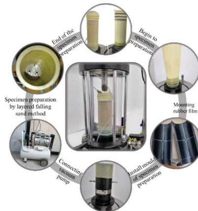
Figure 3. Specimen preparation and specimen installation.
