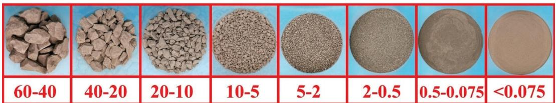
**Figure 2.** Coal gangue particles after sieving tests.
