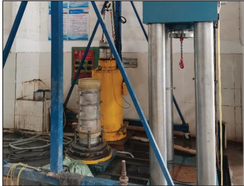
**Figure 3.** The large-scale dynamic and static triaxial instrument.
