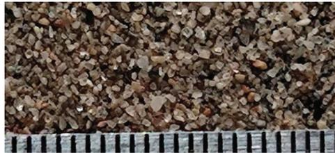
Figure 2. Microscopic image of test material (0.5 mm/grid).
