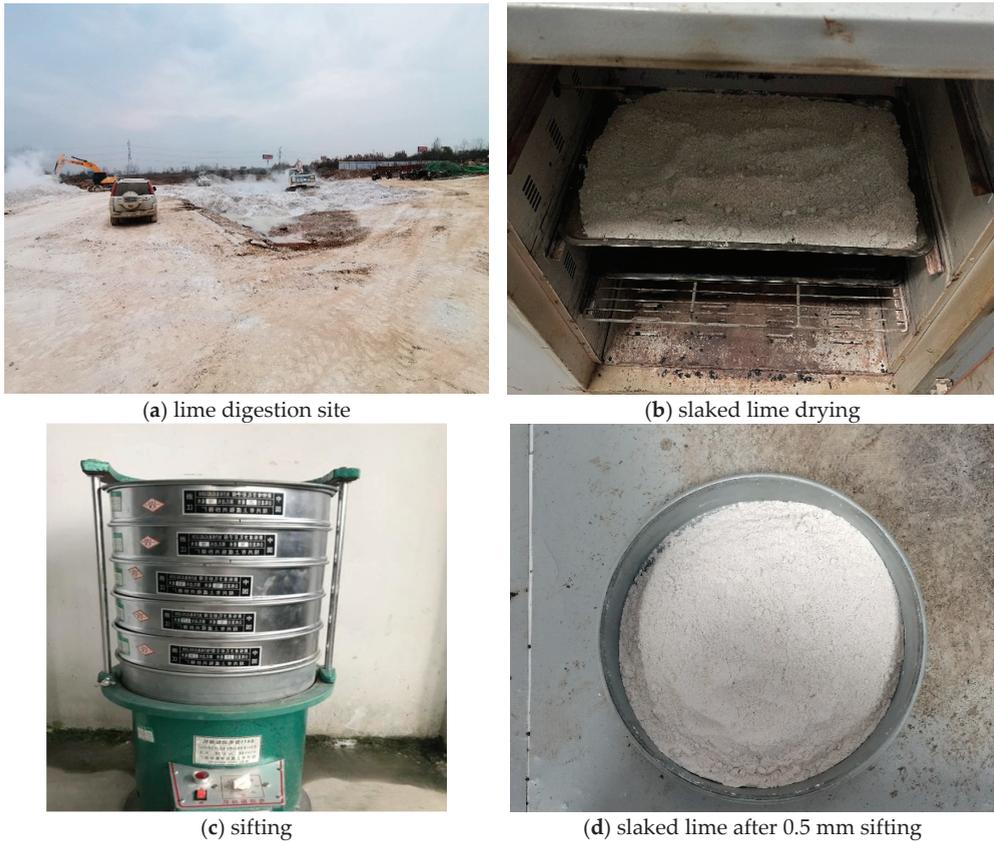
**Figure 3.** Lime preparation for test.
