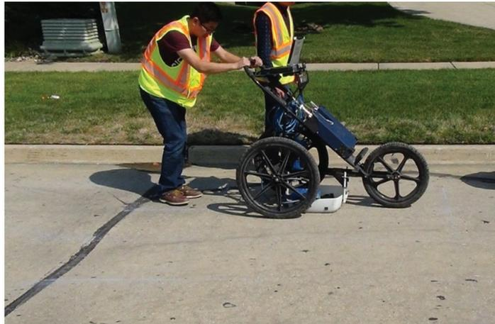
**Figure 3.** GPR survey conducted on a test site.
