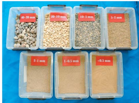
**Figure 2.** Sieved soil material for each grain group.
