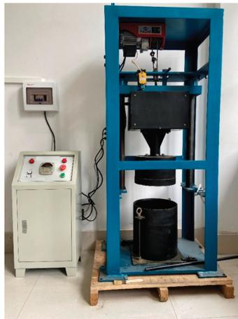
Figure 4. Surface vibratory compactor for coarse-grained soils.
