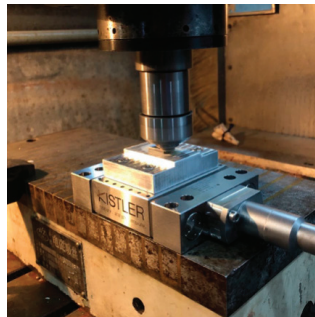
Figure 6. Device diagram of the grinding force experiment.
