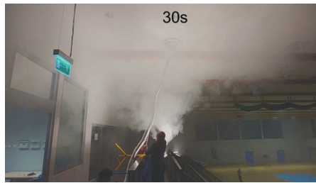
Figure 5. Visualisation of the air stream from the swirl diffuser in the 30th second.
