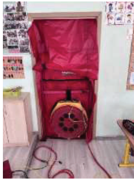
Figure 3. Blower door test.
