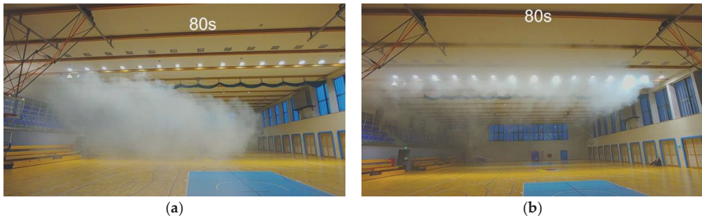
Figure 4. Visualization of the air stream from the nozzle directed downward (a) and upwards (b) in the 80th second.
