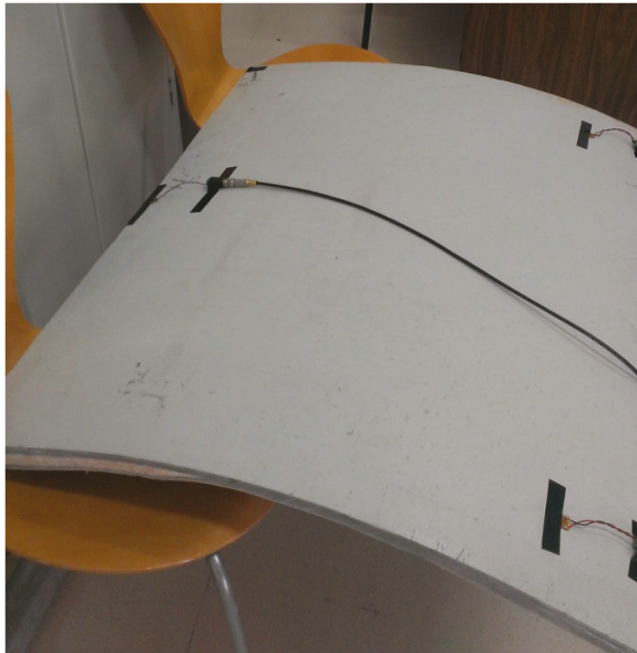
Figure 1. Wind turbine section with sensors for acoustic emission location.
