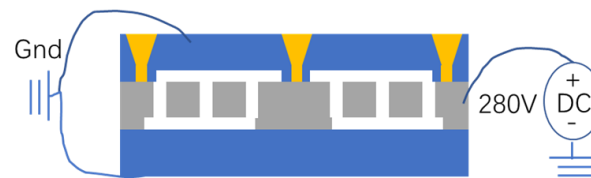
Figure 6. Anodic bonding was used for wafer-level package.
