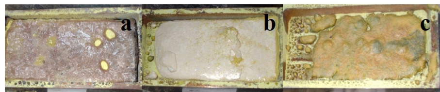
Figure 10. Photographs of ceramic samples (a) \text{ZnWO}_4 , (b) \text{MgWO}_4 , (c) \text{CaWO}_4 , synthesized under the influence of an electron beam with E = 1.4 MeV, P = 18 \text{kW}/\text{cm}^2 , R1.
