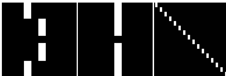
Figure 4. Artificial membrane structures with obstacles in different positions. These three structures are designed to show which distributions of obstacles can cause changes in transport. Left panel: The first structure has three breaks (structure S1). Central panel: The second structure has only one break, at the central point of the membrane (structure S2). Right panel: The third structure has obstacles aligned along the main diagonal of the structure (structure S3). The breaks between the obstacles are equally distributed.
