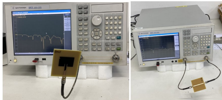
Figure 74. Setups used for the experimental characterization of the microstrip patch and microstrip line with a DGS with open and closed square Matryoshka cells.
