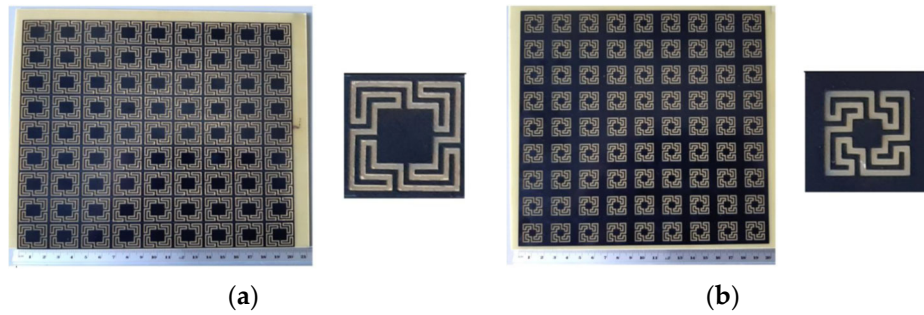
Figure 37. Photos of the prototypes of the complimentary Matryoshka configurations FSS1 and FSS2. (a) FSS1. (b) FSS2.
