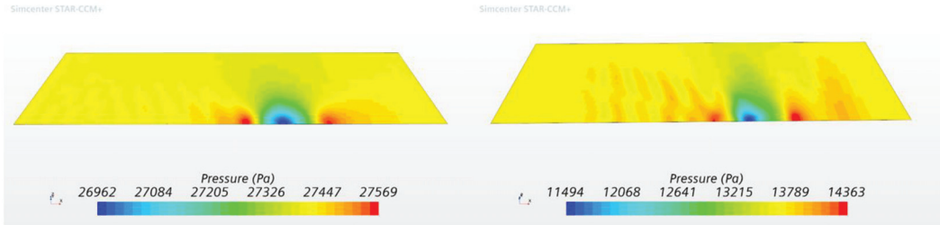
Figure 13. Pressure distribution at the bottom of the computational domain for h/T = 4 (left) and h/T = 2 (right) at a speed of 5.5 knots.
