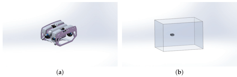
Figure 9. BlueROV2 model. (a) Simplified BlueROV2 geometry; (b) Simulation flow zone.
