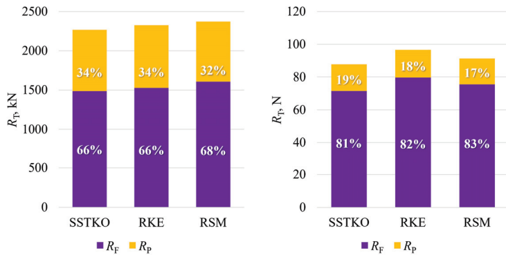
Figure 32. The portions of the total resistance components obtained with different turbulence models within the numerical simulations at full scale (left) and model scale (right).
